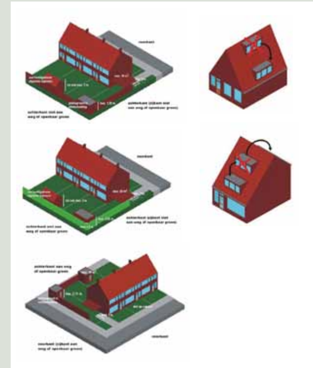
Figure 29. The quality measures that the Neerijnen Welstandsnota envisages are illustrated with schemes and drawings, with all the necessary notes so that owners and builders can follow them. The features that are regulated include the layout of constructions, gardens, courtyards and even windows, among others.
