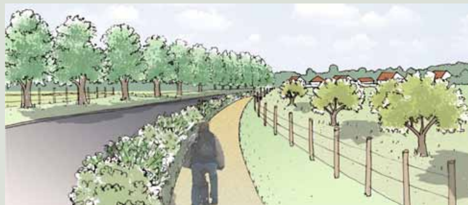
Figure 16. Example of diagram which illustrates the planning proposal for the 922 route (between Mortefontaine and Plailly), with the planting of rows of pear trees, a new lower strip of bushes between the road and the bicycle lane and the replacement of the horticulture plants for fruit trees in the interior of the plot.
