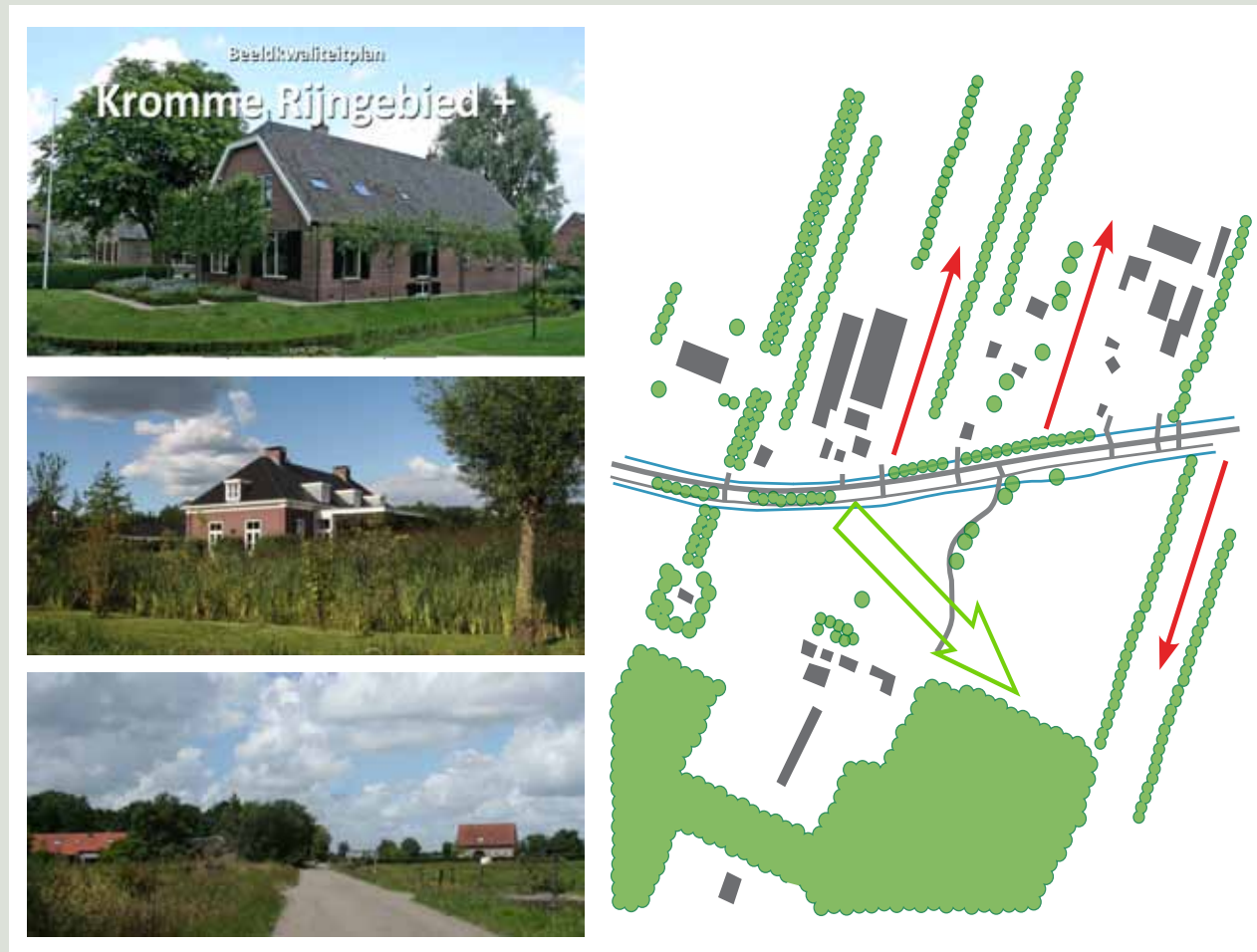
Figure 27. Diagram of the representation of a specific sector of the territory in the Kromme Rijn Landscape Quality Plan (with images of existing features on the left). It can be seen how the constructed features, as well as the natural ones are represented, and the relationship between them in order to give an idea of the configurations of the landscape as a whole.
