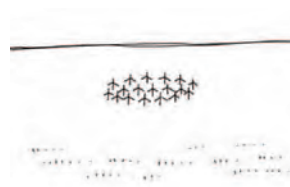
Where a landscape does not include any obvious elements or features to which a windfarm could relate directly, it may be most appropriate for a windfarm to form a distinct feature in its own right. However, for this approach to appear clear, it will usually require the windfarm to be surrounded by an area of open space.
