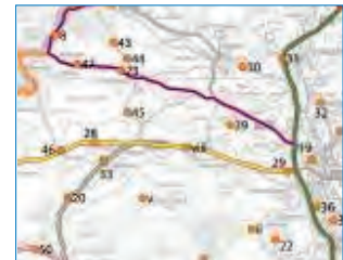
Plan showing sample viewpoint locations that informed the development of a windfarm capacity study. For each viewpoint, site assessment was carried out in addition to the production of visualisations that showed sample wind turbines of different height in various hypothetical locations in relation to the viewpoints across the region.
