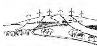
Visual link between windfarm and elements of known size, aid perception of scale and distance, emphasising the height of the wind turbines
