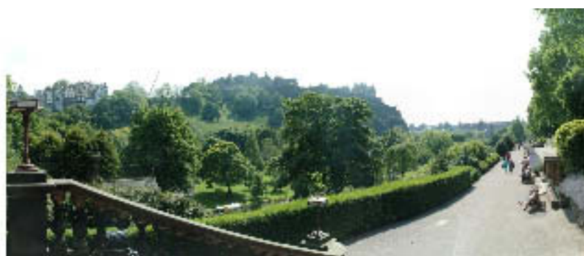
Figure B17: Cylindrical panorama with a horizontal field of view of 106^\circ . This is the type of image produced by a rotating lens panoramic camera or by splicing together single frames from a conventional panorama. The horizontal scale is the same across the whole width of the image. The viewing distances for both panoramas are the same, so the scales are equal in the centre of the planar panorama.
