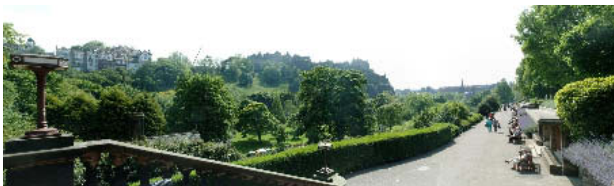
Figure B16: Planar panorama with a horizontal field of view of 106^\circ . This is the type of image produced by a fixed-lens panoramic camera and is equivalent to an extreme wide-angle single frame. The increase in image scale towards the sides of the image are very apparent.
