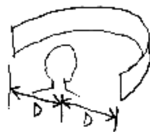
Figure B14: A cylindrical panorama can be superimposed on the scene when viewed from the centre of curvature of a curved surface whose radius is the correct viewing distance.
