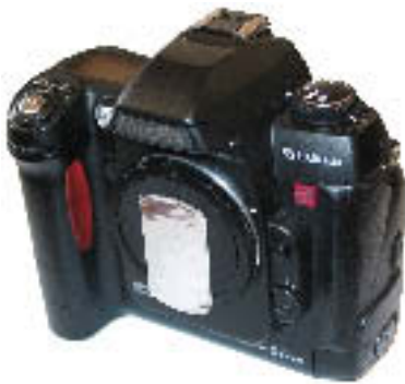
Figure A3: A pinhole camera improvised by replacing the lens of a digital SLR with a modified body cap.
