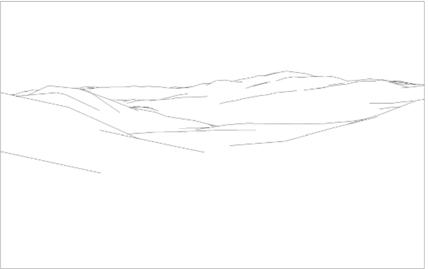
Wireline drawing of OS Panorama DTM at the supplied 50m grid size
